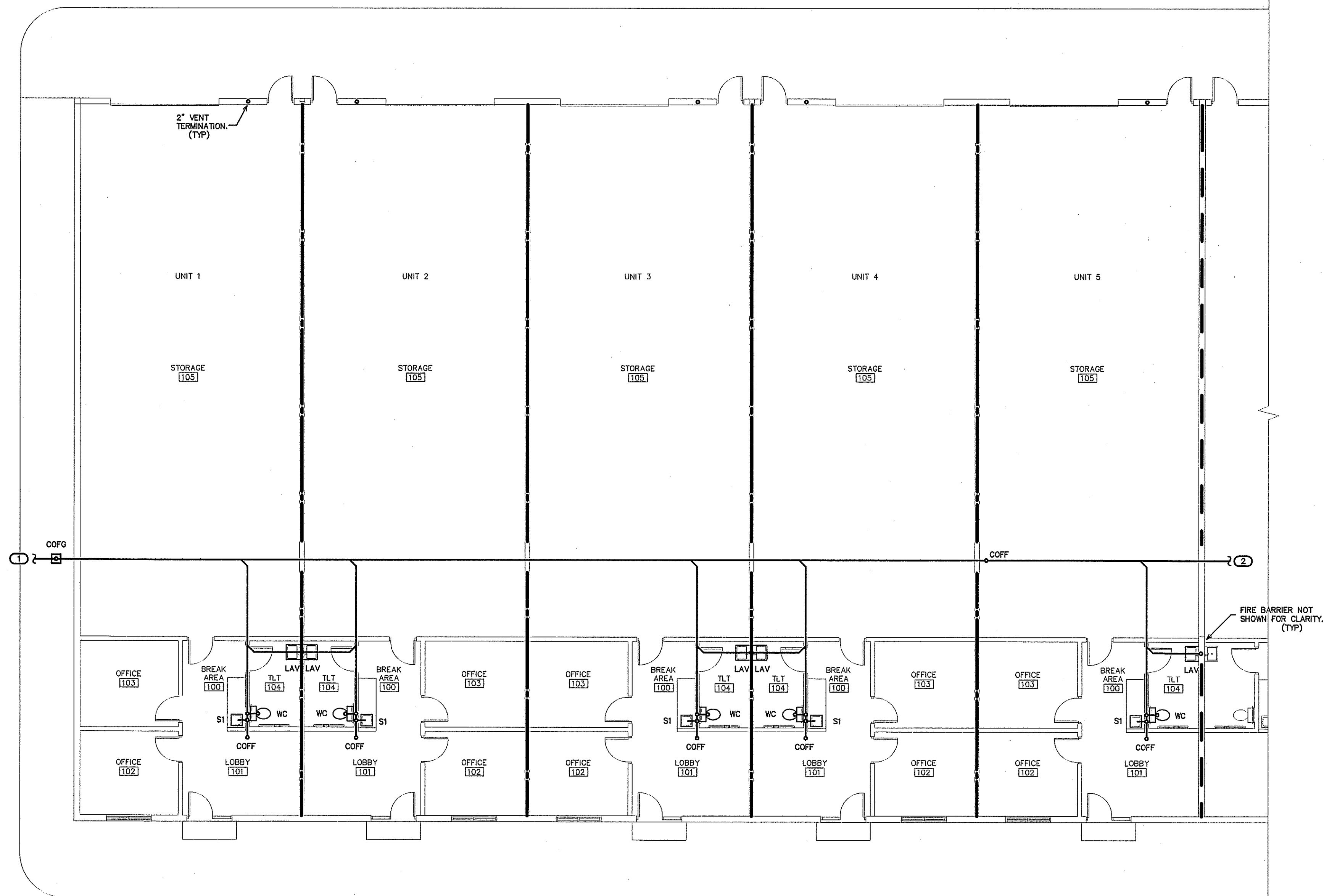
1 DWV PLAN - SIDE A P2.0 SCALE: 1/8"=1'-0"
